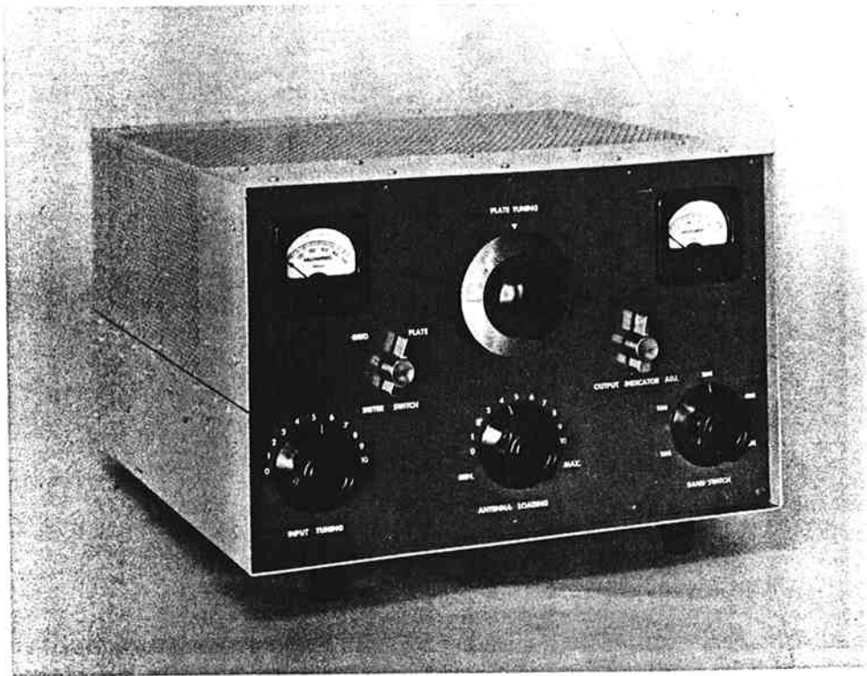
Figure 1. 3-400Z grounded grid amplifier runs 1 kw PEP input on all amateur bands between 10 and 80 meters, with a distortion figure better than -35 decibels below maximum output. Amplifier is enclosed in TVI-proof cabinet.
